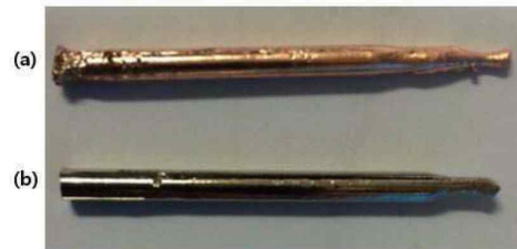
(a) (\text{Fe}_{76.5}\text{Nb}_{8.5}\text{B}_{15})_{70}\text{Cu}_{30} : 황동색 (b) (\text{Fe}_{76.5}\text{Nb}_{8.5}\text{B}_{15})_{93}\text{Cu}_7 : 회백색
